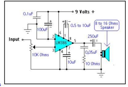
capacitor is shunted in parallel with another one of 0.1uF. It can be either ceramic or mylar.
