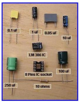
The picture to the left is all of the components used in the LM386 audio amplifier project.
