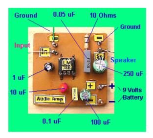
The LM386 IC has been designed to work with low voltages...between 4 to 15 volts. The current taken from the power source or the batteries when standing by, is also quite small, something around 3 mA's. If you add to these qualities the possibility of changing the amplification power, you realize that the LM386 chip is an attractive circuit to work with.
